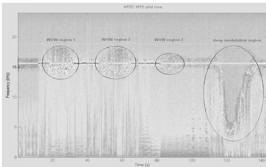
Figure 3: Wow-distorted audio sample spectrogram
