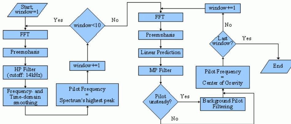
Figure 2: Block diagram of the MTS tracking algorithm
