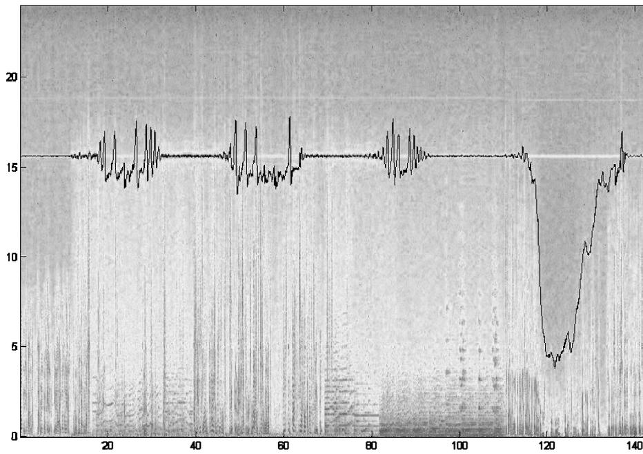
Figure 5: Wow-distorted audio sample spectrogram with tracked MTS pilot tone
