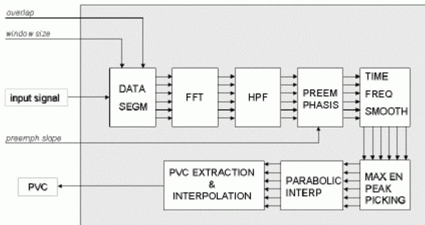
Figure 1: Block diagram of the HFB tracking algorithm [2]
