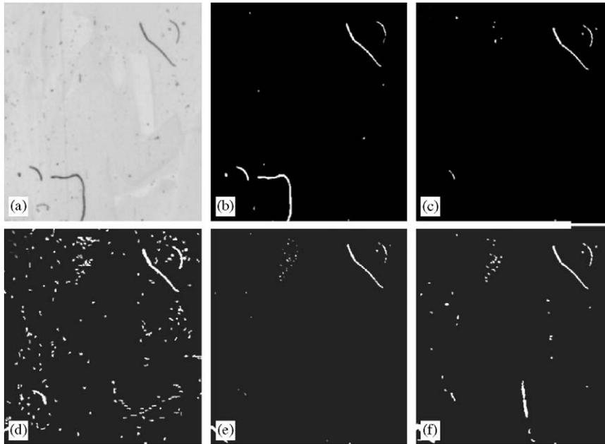
Fig. 7. Comparisons of GT and detected dirt for the image Fig. 5(a). (a) Gray-level GT map of dirt, (b) binary GT of dirt at threshold = 80, (c) detected dirt using SDIp with  $t_2 = 10$ , (d) detected dirt using ROD,  $t_1 = 3$ ,  $t_2 = 6$ ,  $t_2 = 10$ , (e) detected dirt using LUM (27,9) with  $t_s = 10$  and (f) detected dirt using ML3Dex with  $t_s = 10$ .
